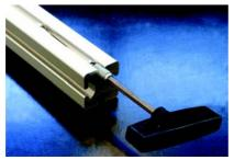
Screw-in the Automatic Fastener using the key with T-handle (or cordless screwdriver) into the groove. The Automatic Fastener cuts a thread inside the profile's groove.
