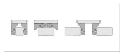
The roller profiles provide a variety of fastening options using the grooves of Line 8 Profiles, this greatly simplifying installation and alignment on profiles or carriage plates.
