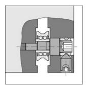
The eccentric bearing units must be set prior to the guide carriage being used:
