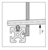
With longer sections where the support profiles have already been installed or are held in a vice, for example, it is possible after inserting the Shaft-Clamp Profile to press the Shaft into the latter progressively, starting at one end by using the Mounting Aid (Order No. 0.0.265.38) and an appropriate round steel bar as a lever.
