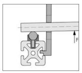
On longer stretches, when the support profiles have already been installed or are being held in a vice and the Shaft-Clamp Profile has been pressed into place, you can press the shaft into the Shaft-Clamp Profile section by section using the Mounting Aid (0.0.265.38) and a lever in the form of a suitable round steel bar.
