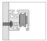
When higher loads are involved, it is advisable to secure the Shaft. Ideally, a Combination Drilling Jig c should be used to machine the Shaft. Shaft-Clamp Profile and Support Profile as detailed in the following steps:
