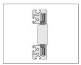
To construct a linear guide, two centric (fixed) and two eccentric (adjustable) bearing units are normally required. Each pair of single bearing units can be replaced by one double bearing unit.
