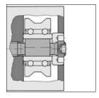
You must prepare the eccentric orientation of the eccentric Bearing Units before using the guide carriage. Use an Allen key to turn the eccentric bolt of the rollers:
