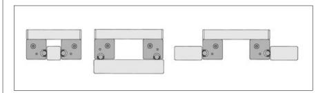
The roller profiles provide a variety of fastening options using the grooves of Line 8 Profiles, this greatly simplifying installation and alignment on profiles or carriage plates.
