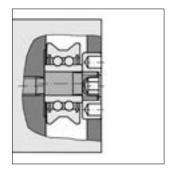
The eccentric bearing units must be set prior to the guide carriage being used. The Allen key drives in the rollers' eccentric bolt:
