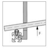
With longer sections where the support profiles have already been installed or are held in a vice, for example, it is possible after inserting the Shaft-Clamp Profile to press the Shaft into the latter progressively, starting at one end by using the Mounting Aid (Order No. 0.0.265.38) and an appropriate round steel bar as a lever.
