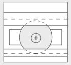
C-Rail System K with slide consisting of plastic rollers running directly on the aluminium rail profile. This variant can accommodate low hanging loads as shown in the illustration opposite and is adequate for simple guide operations.
