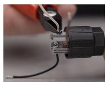
Now insert the strands according to their colour into the colour-coded, numbered clamps in the connector, press them down and fix them in place. Use a side cutter to separate the wires directly at the outer edge.
