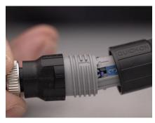
Manually screw the second part of the connector onto the lower part of the plug, aligning the arrows on each half of the connector.
