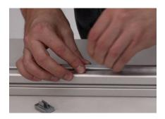
Slide the free end of the Cap outwards and remove it from the Profile. Release the LED Casing Profile from the clamp in the aluminium Profile.
