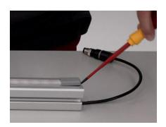
Lever out the Cap on the cable with a screwdriver.
