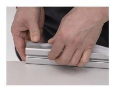
Carefully press the casing profile containing the LED strip manually into the groove of Profiles 8 along with the Cap. In doing so, the Cap should be aligned with the cut edge of the profile.
