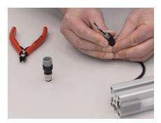
Feed the cable through the connector until the outer insulation disappears into the connector and you hit a limit stop.
