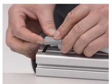
Now press the Cap with its clamping bars over the white protective cover of the protruding cable and push it over the casing profile until the clamping bars rest on the profile.
