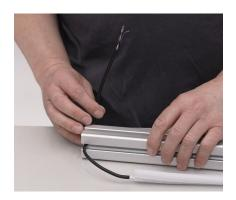
Feed the cable through the hole in the profile.
